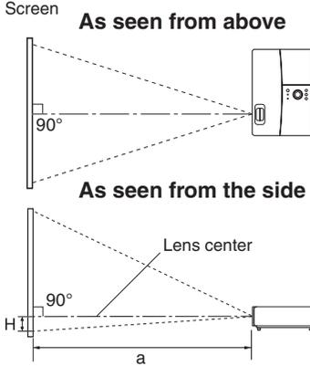
**a** is the distance (m, feet) between the lens and the screen, and corresponds to a range of 0.89 m (2.92 ft.) to 10.93 m (35.86 ft.). **H** is the height from the image bottom to the center of the lens.
