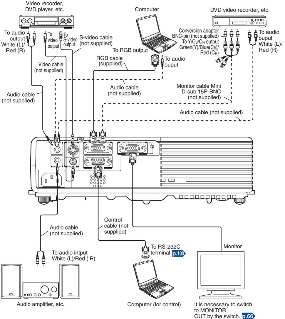
\* The connection for COMPUTER 1 IN terminal described here is also applicable for COMPUTER 2 IN terminal.
