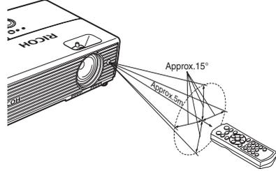
When operating the remote control from behind the projector, the infrared signal is reflected on the projecting surface and may travel a shorter distance to reach the projector depending on the shape and material of the projecting surface.
