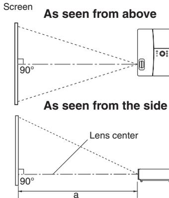
**a** is the distance (m, feet) between the lens and the screen, and corresponds to a range of 0.94 m (3.08 ft.) to 11.58 m (37.99 ft.). The lens center is in the same level with an image bottom.
